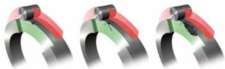
Formation of damage on the surface
