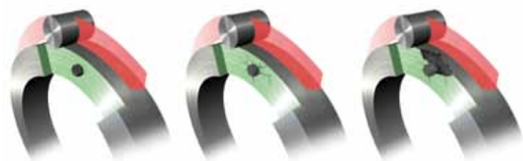
Formation of damage below the surface
